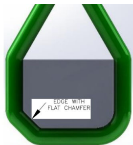
Figure 29 Inappropriate Direct Contact of Unprotected Roundslings with a Chamfered Edge
